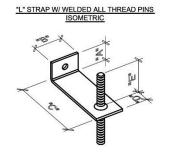
Typical "A" dimensions are 1"-2". Typical "B" dimensions are 1"-2". Typical "C" dimensions are from center of stone to the face of sheathing/outside face of wall structure. Typical "D" dimensions are  $\frac{3}{4}$ "-1".
