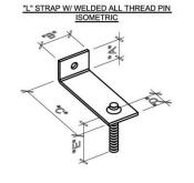
Typical "A" dimensions are 1"-2". Typical "B" dimensions are 1"-2". Typical "C" dimensions are from center of stone to the face of sheathing/outside face of wall structure.
