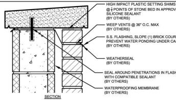
@ 1 POINTS OF STONE BED IN APPROVED SILICONE SEALANT (BY OTHERS) · WEEP VENTS @ 36" O.C. MAX (BY OTHERS) S.S. FLASHING, SLOPE (1) BRICK COURSE TO PREVENT WATER PONDING UNDER CAST STONE (BY OTHERS) WEATHERSEAL (BY OTHERS) SEAL AROUND PENETRATIONS IN FLASHING WITH COMPATIBLE SEALANT (BY OTHERS)
